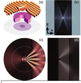
Transformation optics devices: a): cloak, b): light concentrator, c): impedance-matched hyperlens, and d): planar hyperlens
