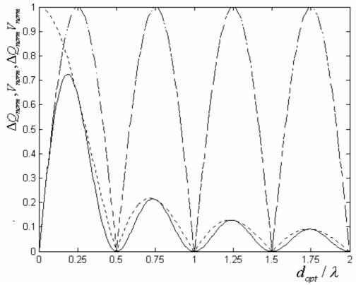
Fig.2. Interference signal of a photodetector  $\Delta Q_{norm}$  (dash-dotted line), contrast  $\varsigma_{vo\rho\mu}$  (dashed line),  $\Delta Q_{norm}V_{norm}$  (continuous line). On an abscissa axis the normalized optical distance of a photoelectric stratum is postponed. The total response of a photodetector is proportional:
