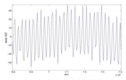
Fig. 5. Response of a photodetector at its uniform driving in an interferential field of counter luminous fluxes He-Ne of the laser.
