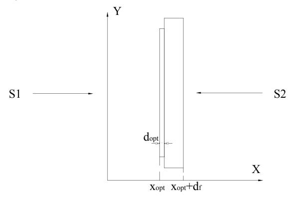
Fig.1. Arrangement photodetector and optical axis position data.
