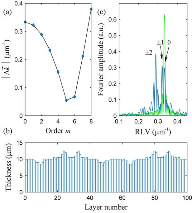
Fig. 3. (a) Absolute value of the wave vector mismatch versus the transverse QPM order. (b) Layer thickness as a function of the layer numbers in the direction  $y$ . (c) Reciprocal lattice vector spectra of the periodic (green) and aperiodic (blue) function  $\eta(y)$ .
