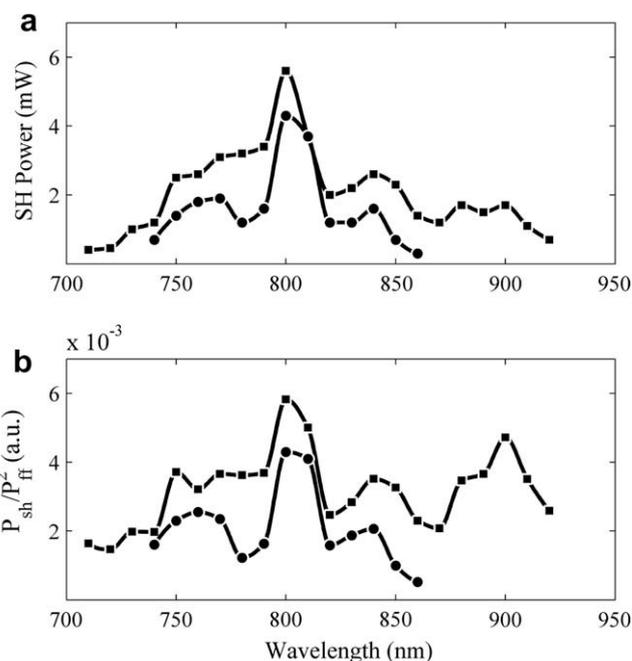
Fig. 2. (a) Spectral dependence of second harmonic power by tuning the femtosecond Ti:sapphire oscillator; (b) RSV spectrum of SBO nonlinear photonic crystal; squares – with translational tuning of second harmonic, circles – for fixed position of the beam.
