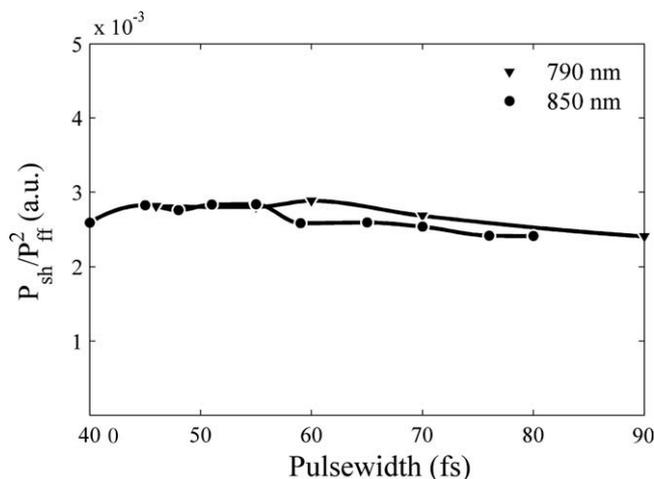
Fig. 4. Variation of second harmonic coupling coefficient with the duration of the fundamental pulses at the entrance of nonlinear medium.
