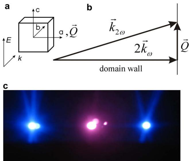
Fig. 1. (a) Geometry of fundamental wave propagation; (b) phase matching diagram; (c) nonlinear diffraction pattern of second harmonic radiation from SBO. The fundamental wavelength is 800 nm, with average power 1 W.
