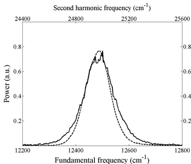
Fig. 3. Spectra of fundamental (solid line) and second harmonic (dashed line). Ocean Optics HR4000, resolution 0.75 nm.
