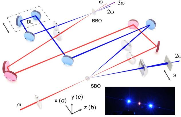
Fig. 1. Experimental setup for studying CND in the frequency (lower stage) and time (upper stage) domains (S, adjustable-width slit; DL, delay line). Domain walls lie in the crystallographic plane  $bc$ . Inset (bottom right): CND pattern on the screen.
