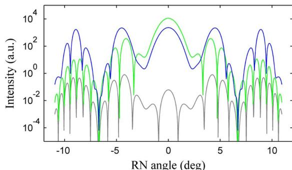
Fig. 5. Resultant angular dependences of second harmonic intensity at the exit from 1D (gray), periodic (green), and aperiodic (blue) 2D nonlinear photonic lattices shown in Fig. 1.
