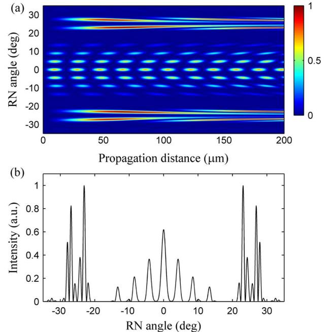
Fig. 2. Angular dependence of second harmonic intensity as a function of (a) the propagation distance and (b) the angular distribution of the second harmonic intensity at the distance  $L = 200 \mu\text{m}$  in a 1D nonlinear photonic lattice.
