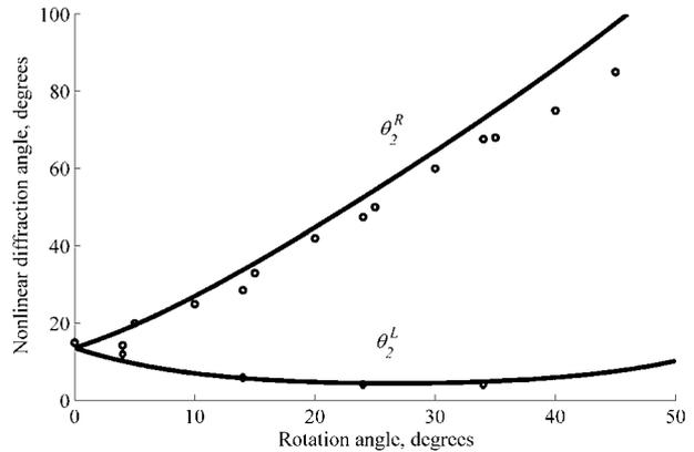
**Figure 2.** Dependence of nonlinear diffraction angles upon crystal rotation angle. Solid lines are calculations, circles and diamonds are the experimental data obtained for the right-hand beam and for the left-hand beam, respectively.
