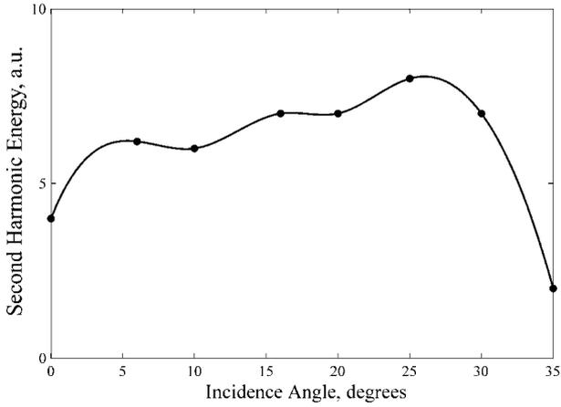
**Figure 3.** Dependence of diffracted second harmonic energy upon incidence angle.  $\theta_1 = 0$  corresponds to  $Q^{L,R} = \pi \mu\text{m}^{-1}$ , and  $\theta_1 = 35^\circ$  corresponds to  $Q^R = \pi/0.22 \mu\text{m}^{-1}$ .
