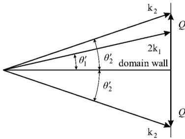
**Figure 1.** Phase-matching diagram for nonlinear diffraction of the second harmonic.
